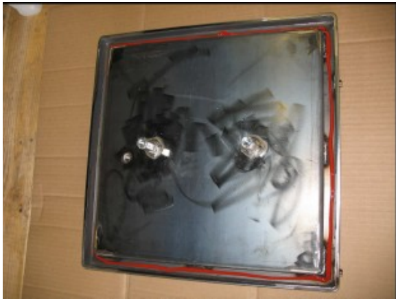
Load Door with Old Seal Removed and High Temperature Silicone
