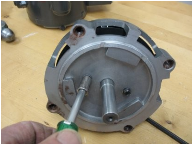
Loosening Screws Securing Bearing to End Shield
