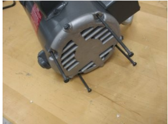
Motor Frame Assembly Bolts
