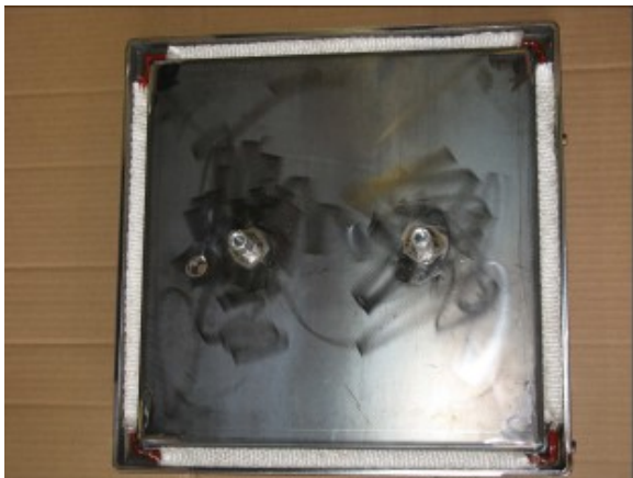
Load Door with Fiberglass Braid Tape
