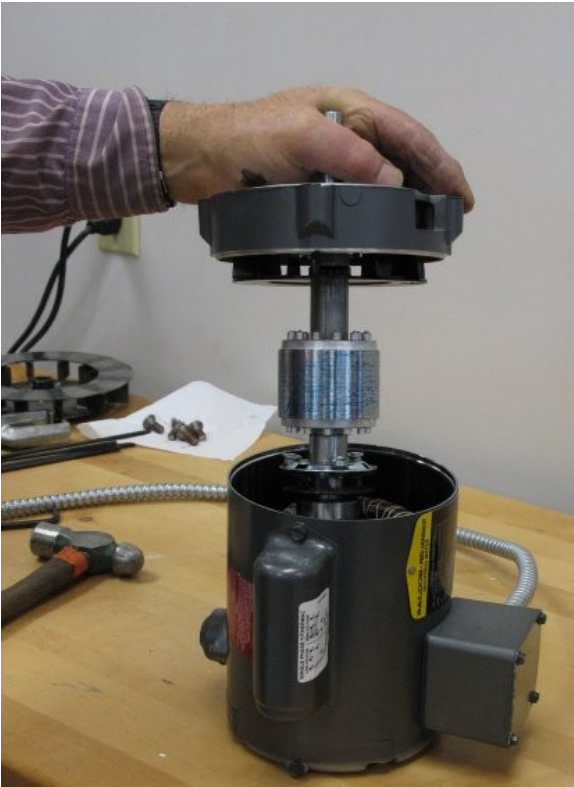
Lifting the End Shield with Armature
