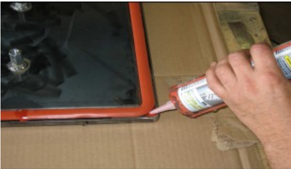
Reinforcing Corners with High Temperature Silicone
