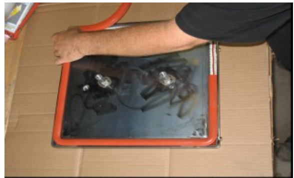
Adding Preformed Silicone Bead to Door
