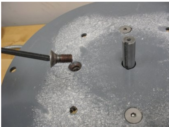
Closeup of Motor Mounting Bolts
