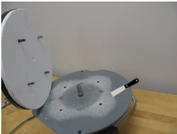
Separate Heat Shield from Motor Mount Plate
