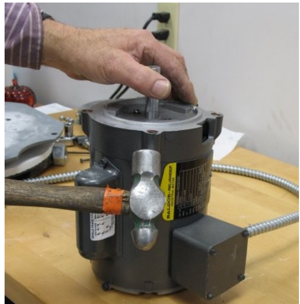
Loosening Motor End Shield from Motor
